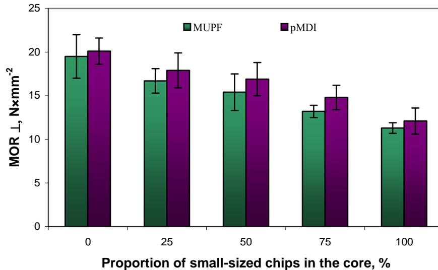
**Fig. 4.** Bending strength of OSB determined for the smaller axis
