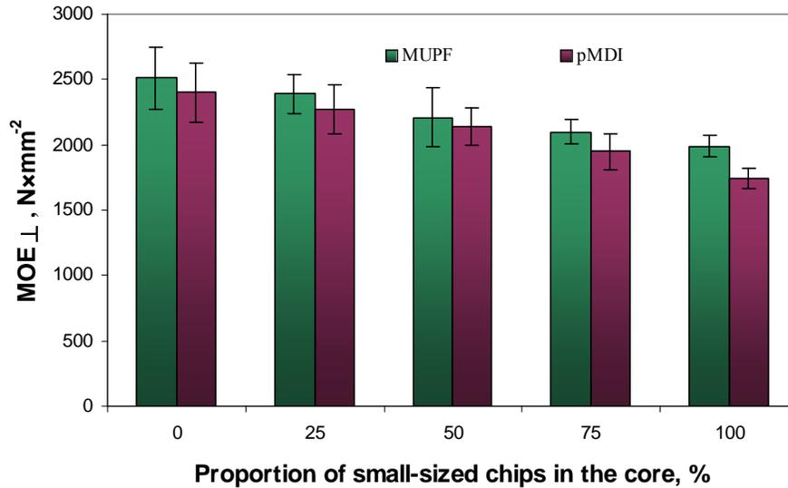
**Fig. 5.** Modulus of elasticity of manufactured OSB determined for the smaller axis
