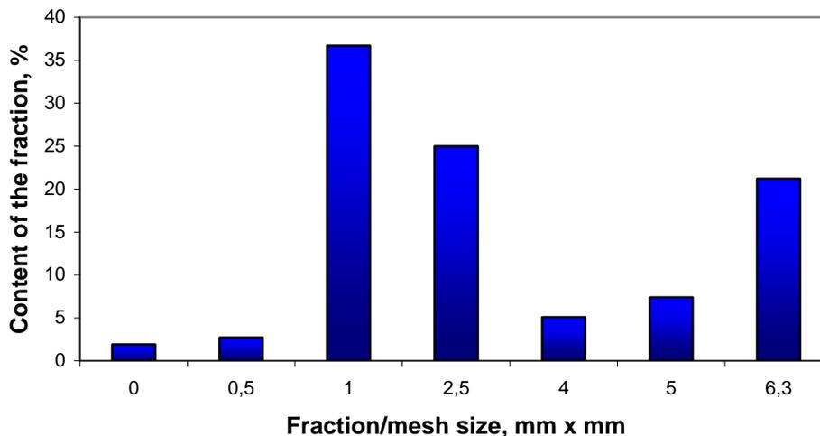
Fig. 1. Sieve fraction of particleboard chips
