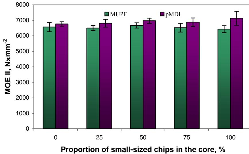
**Fig. 3.** Modulus of elasticity of manufactured OSB determined for the longer axis
