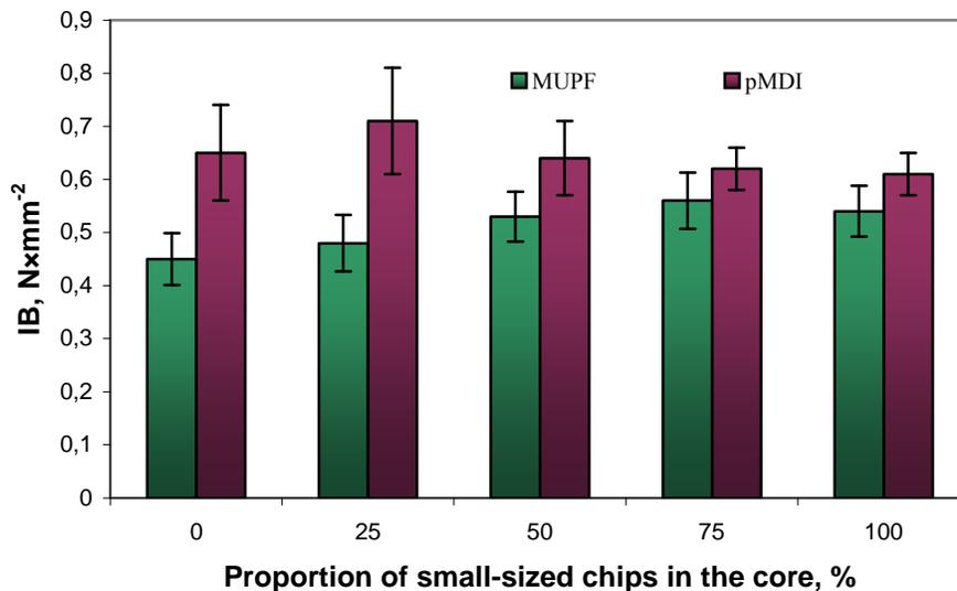
**Fig. 6.** Internal bond of manufactured OSB
