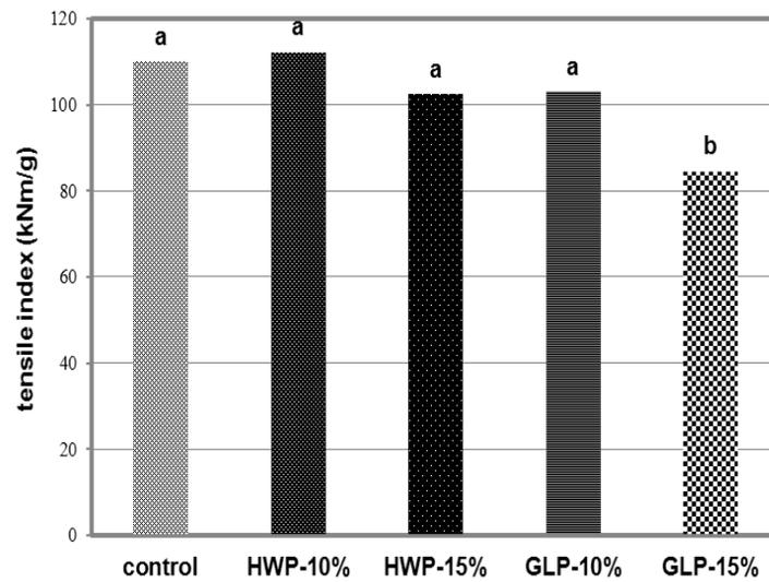
**Fig. 2.** The effects of different pre-extractions on the tensile index in comparison with control pulp
