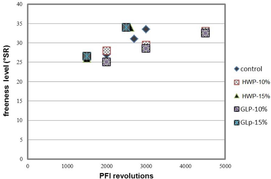
**Fig. 1.** The refining response of the pre-extracted pulp samples versus control pulp. (HWP-10% and HWP-15% stand for pulps pre-extracted with hot water at 10 and 15% weight losses, respectively. GLP-10% and GLP-15% stand for pulps pre-extracted with green liquor at 10 and 15% weight losses, respectively, and control stand for pulp without any pre-extraction)
