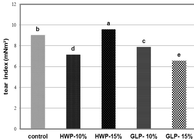
**Fig. 4.** The effects of different pre-extractions on the tear index in comparison with control pulp
