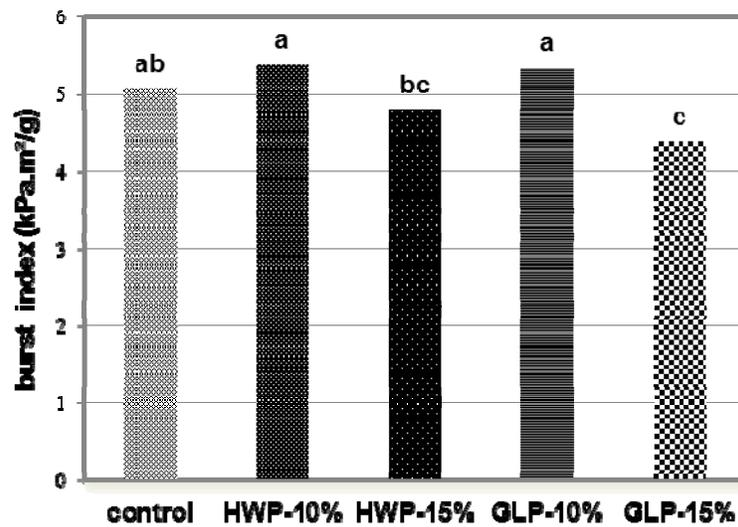
**Fig. 3.** The effects of different pre-extractions on the burst index in comparison with control pulp
