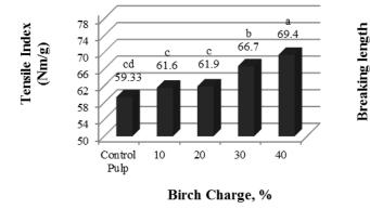
Fig.6. The effect of different charges of birch on pulp tensile index.
