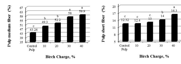
Fig.3. The effect of different charges of birch on pulp medium fiber fraction.
