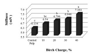
Fig.10. The effect of different charges of birch on pulp stiffness.
