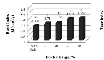
Fig.8. The effect of different charges of birch on pulp burst index.
