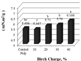
Fig.9. The effect of different charges of birch on pulp tear index.
