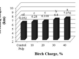
Fig.7. The effect of different charges of birch on pulp breaking length.
