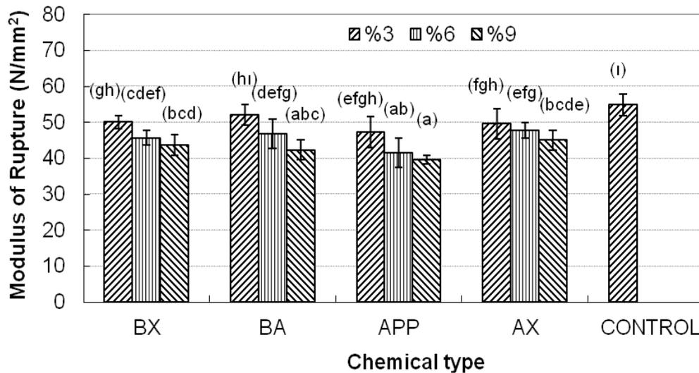
**Fig.3.** Average Values, Statistical Test Results for Modulus of Rupture (MOR) of the HDF Panels Coated with Resin-Impregnated Papers
