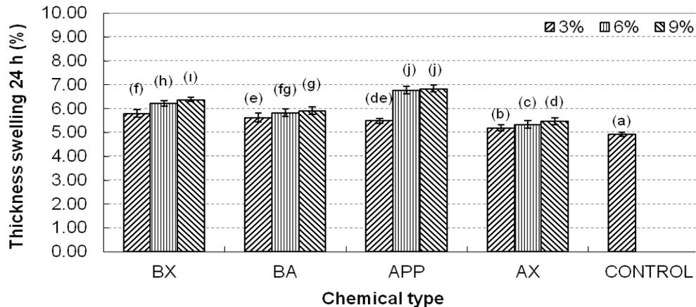
**Fig.2.** Average Values, Statistical Test Results for Thickness Swelling (2h and 24h) of the HDF Panels Coated with Resin-Impregnated Papers.
