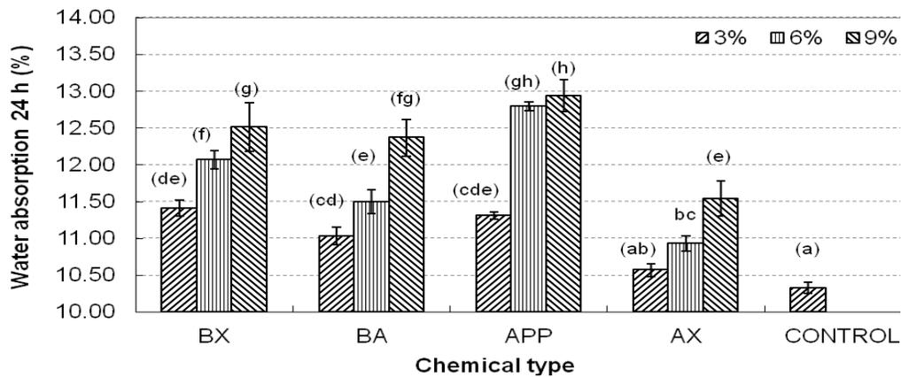
**Fig.1.** Average Values, Statistical Test Results for Water Absorption (2h and 24h) of the HDF Panels Coated with Resin-Impregnated Papers.
