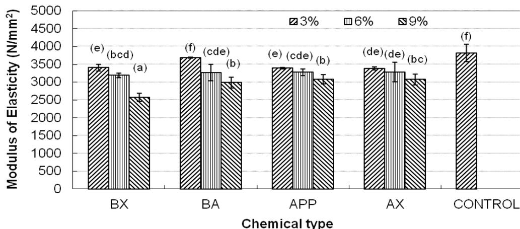
**Fig.4.** Average Values, Statistical Test Results for Modulus of Elasticity (MOE) of the HDF Panels Coated with Resin-Impregnated Papers
