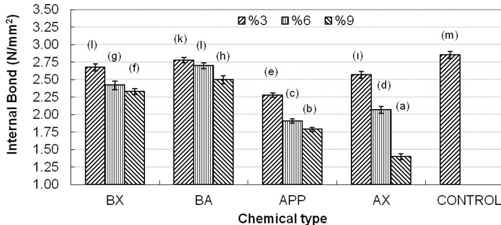
**Fig.5.** Average Values, Statistical Test Results for Internal Bond (IB) of the HDF Panels Coated with Resin-Impregnated Papers
