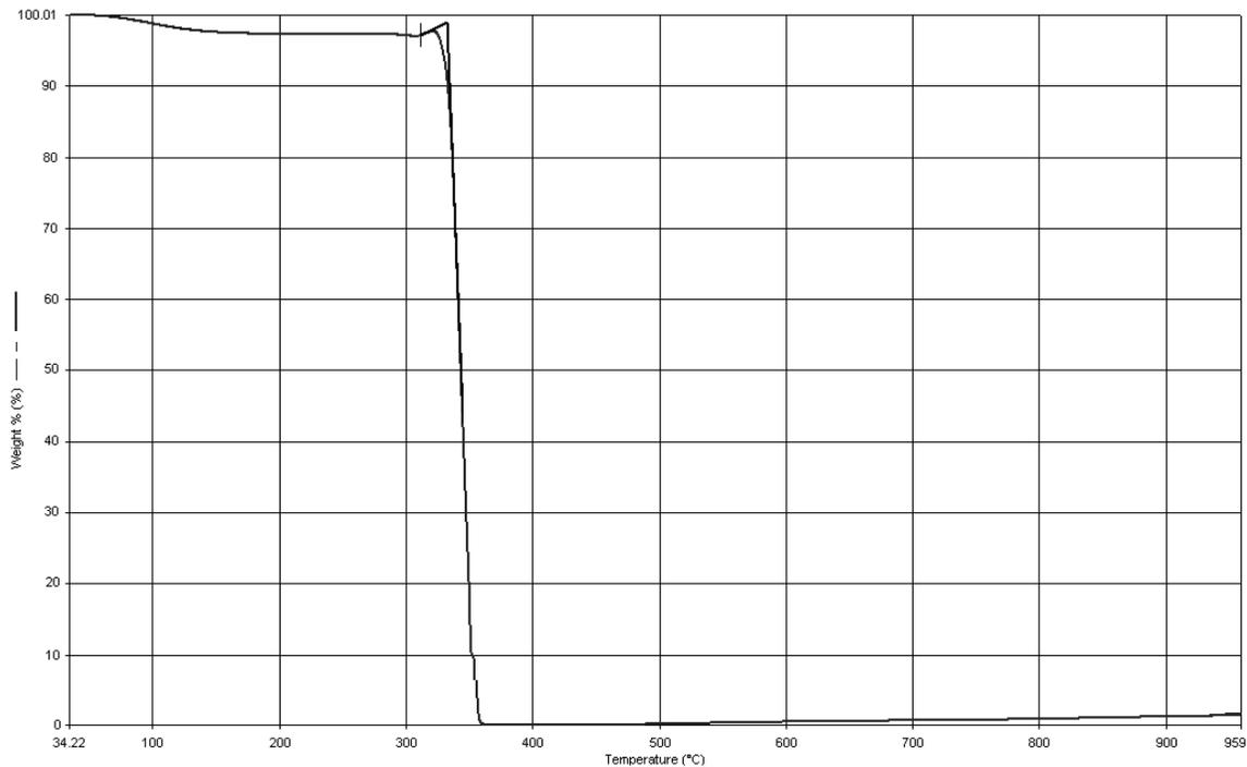
**Fig 4.** Thermo gravimetric analysis of tapioca starch.
