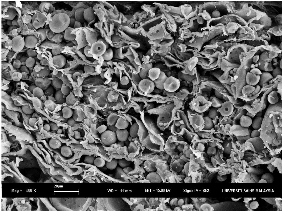
**Fig 1.** Scanning electron microscopy image of starch granules containing in oil palm trunk.
