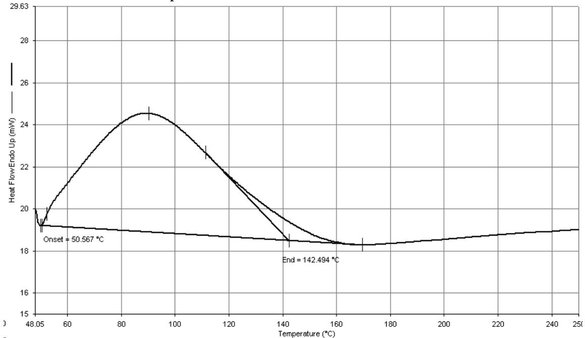
**Fig 3.** Differential scanning calorimetry analysis of tapioca starch.
