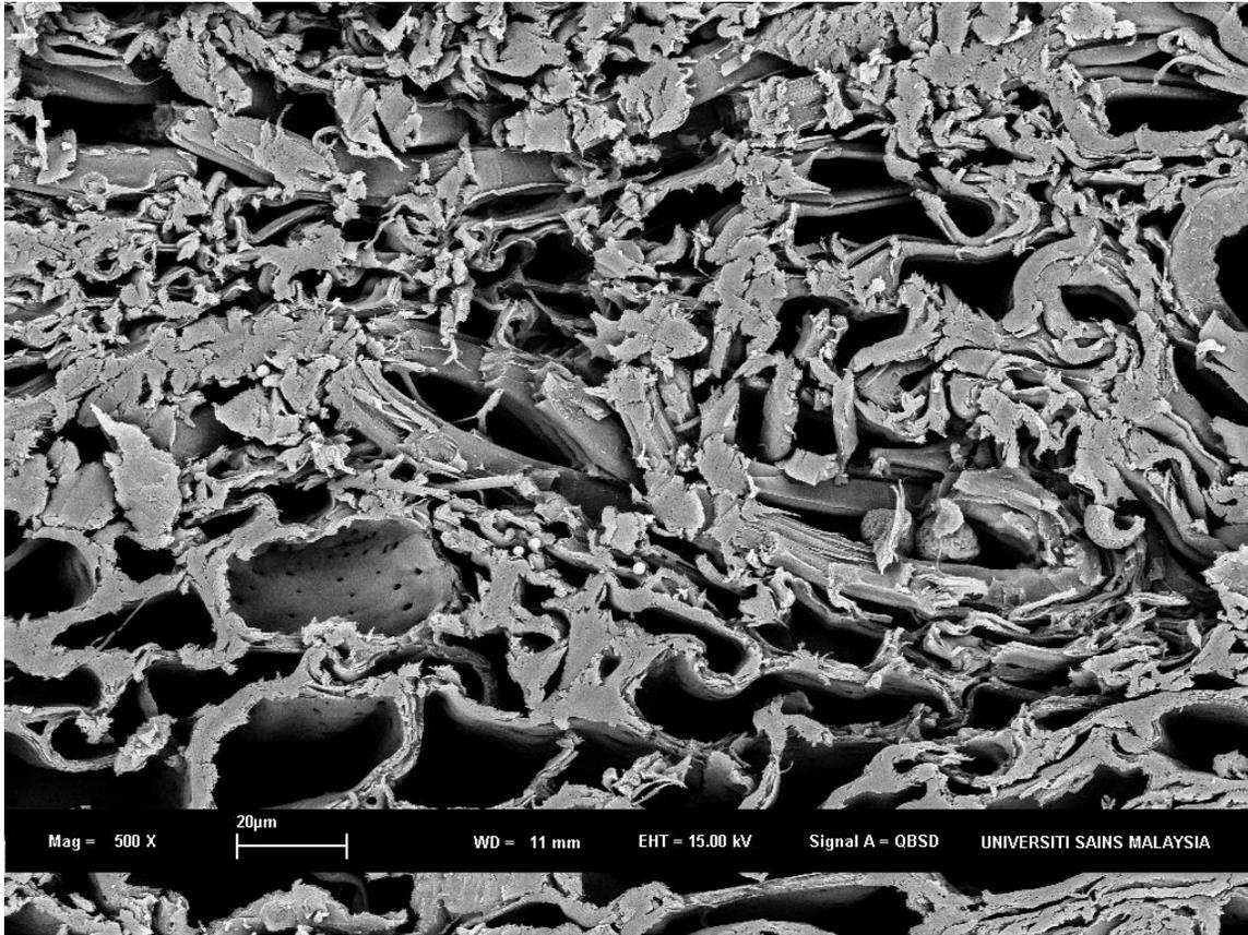
**Fig 2.** Scanning electron microscopy image of specimens made with particles undergone 60 min acid pretreatment.
