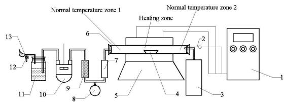
**Fig. 1.** Experimental apparatus. (1) Temperature controller; (2) thermocouple; (3) nitrogen gas tank; (4) porcelain boat; (5) electric furnace; (6) quartz tube reactor; (7) condenser; (8) tar collector; (9) filter; (10) flow meter; (11) water sealed bottle; (12) to gas collector bag; (13) exhaust gas burner.
