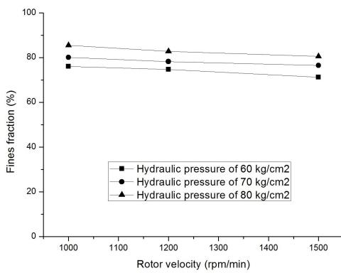
**Fig. 5.** Proportion of the fine fraction ( $d < 90 \mu$ m) in the product as a function of rotor velocity and hydraulic pressure
