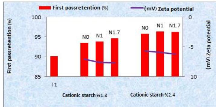
**Fig. 2.** The effect of different Nano-silica (N) and cationic starch treatments on the values of zeta potential and the first pass retention.
