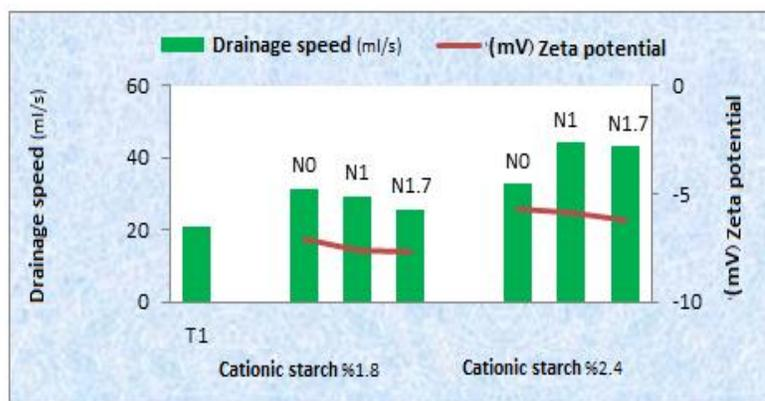
**Fig. 3.** The effect of different Nano-silica (N) cationic starch treatments on the values of zeta potential and drainage ability
