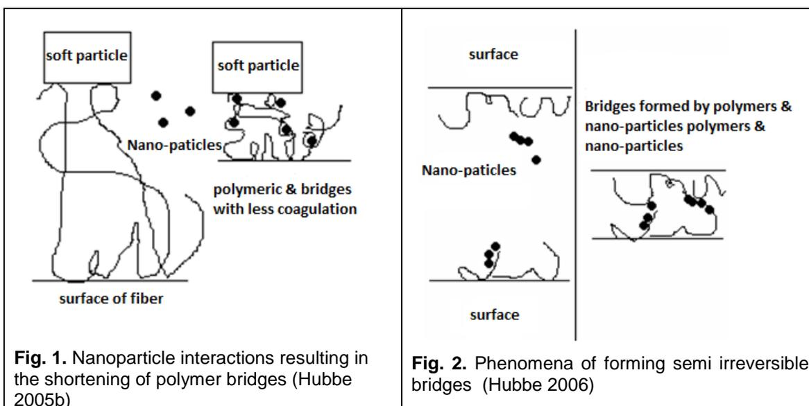
**Fig. 1.** Nanoparticle interactions resulting in the shortening of polymer bridges (Hubbe 2005b)
