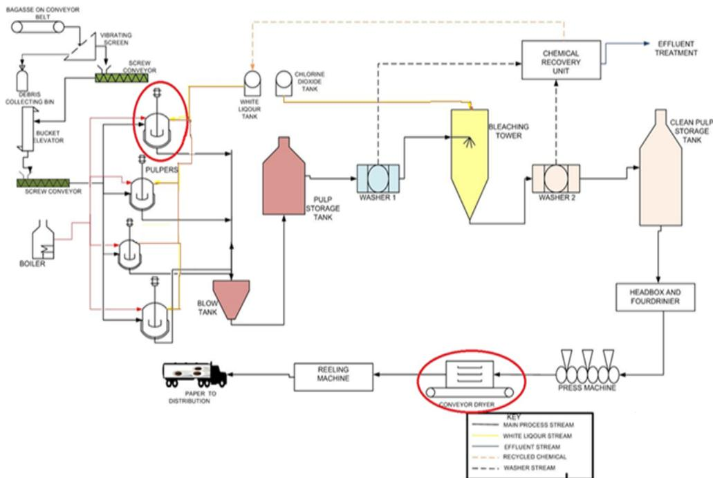
Fig. 5. Process flow diagram for virgin paper processing plant from bagasse
