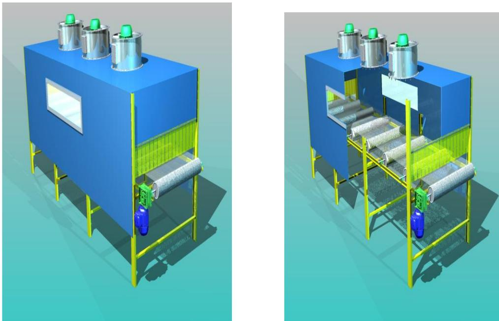
**Fig. 8.** Conveyor dryer (a) South east view, (b) Section view drawn in AutoCad 3
