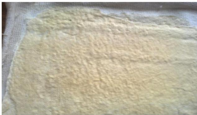
**Fig. 2.** Raw non-virgin paper produced from sugar cane bagasse in the laboratory
