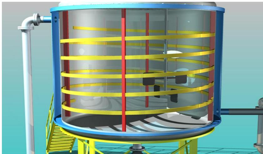
**Fig. 7.** Stirred batch pulper with cross section showing position of agitator drawn in Autocad 3
