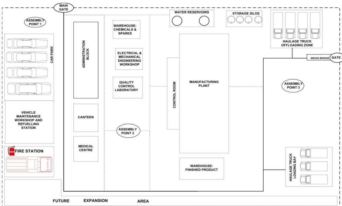
Fig. 9. Plant layout for bagasse virgin paper processing plant
