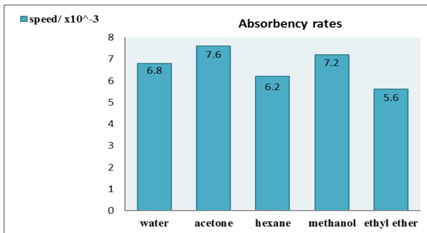
**Fig. 3.** Capillary action results indicating paper absorbency**Determination of Residence Time in Pulper through the Electrical Conductivity**
