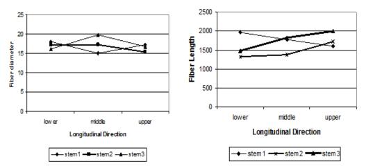
Fig. 3. Fiber length and diameter variation in the bamboo culm
