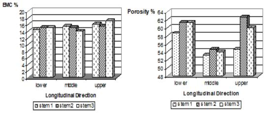
Fig. 5. EMC and porosity variations in the bamboo culm
