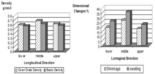
Fig. 4. Density and dimensional change variations in bamboo culm
