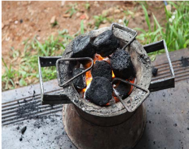
Fig. 1. Charcoal briquettes from agricultural waste
