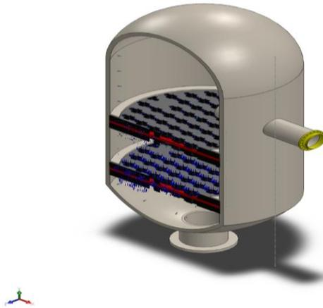
Fig. 5. Cross-sectional view of the adsorption column
