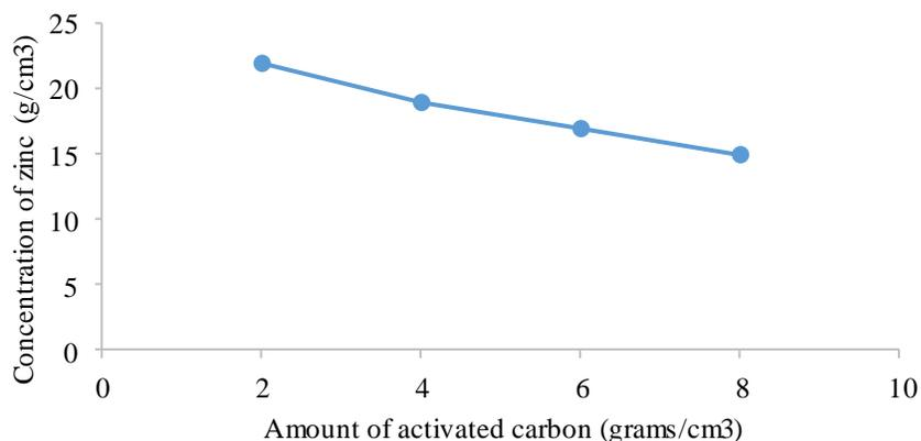
**Fig. 3.** Amount of zinc ions removed for varying activated carbon content
