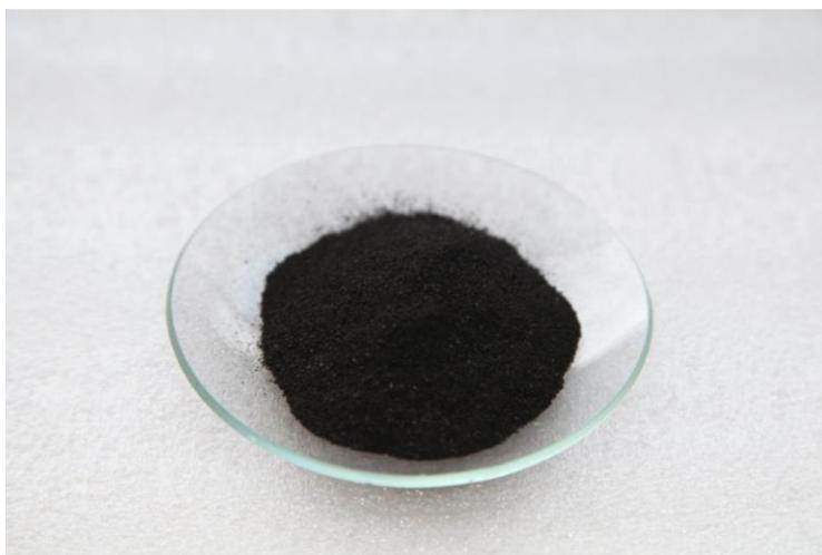
**Fig. 2.** Bio-charcoal from maize corn stover used for zinc ions removal
