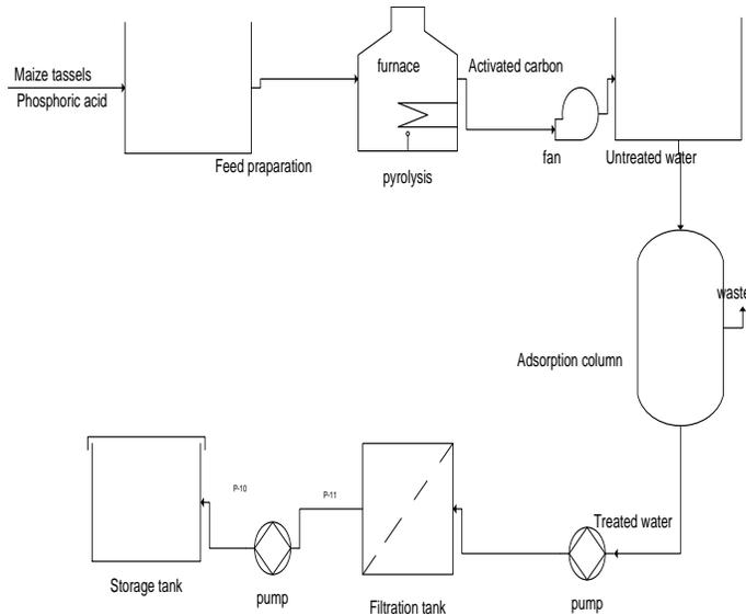
**Fig. 4.** Industrial process design for zinc ions removal using activated carbon from maize corn stover bio-charcoal
