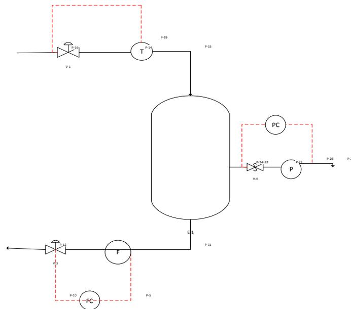
**Fig. 6.** Process control over the adsorption column
