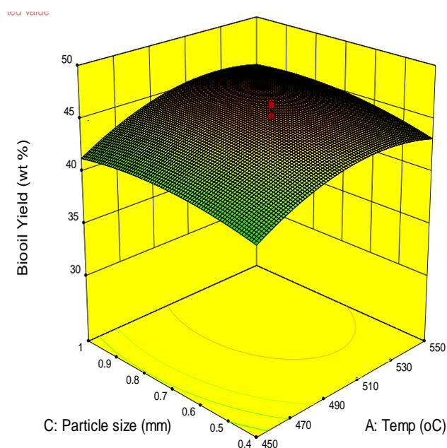
**Fig. 4.** Bio-oil yield as a function of temperature and particle size
