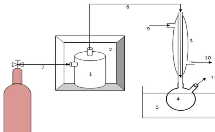
**Fig. 1.** Schematic of experimental set-up: 1. Reactor, 2. Furnace, 3. Reflux condenser, 4. Bio-oil collector 5. Ice trap, 6. Nitrogen bottle, 7. Inert/sweep gas inlet, 8. Vapor outlet 9. Cooling water inlet, 10. Hot water outlet, 11. Non-condensable gas outlet
