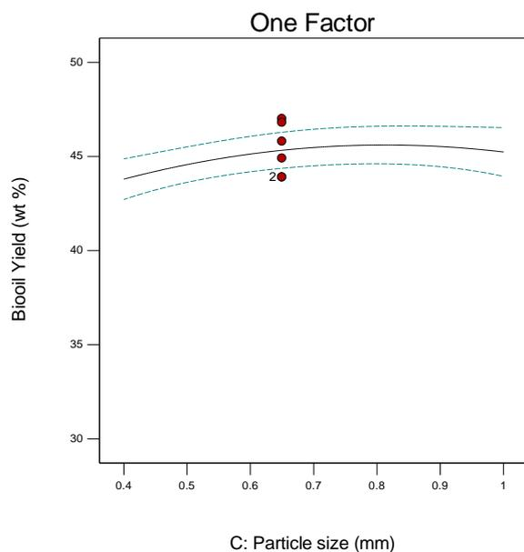
**Fig. 3.** Effect of particle size on bio-oil yield
