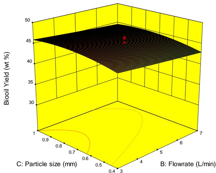
**Fig. 7.** Bio-oil yield as a function of flow rate and particle size
