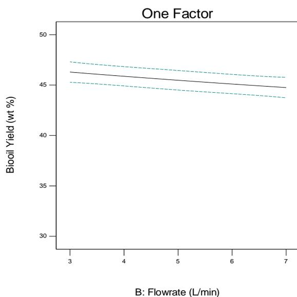
**Fig. 6.** Effect of gas flow rate on bio-oil yield
