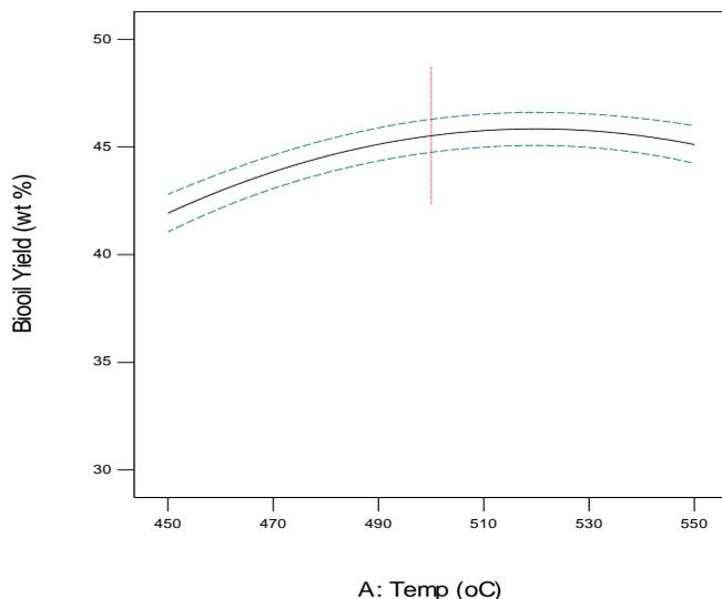
**Fig. 5.** Effect of temperature on bio-oil yield
